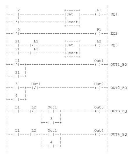
Rung L1 is equation 1. It latches on when the start button is true and unlatches when the NC stop button is pushed. The latch remembers start and stop commands to simplify the logic.
